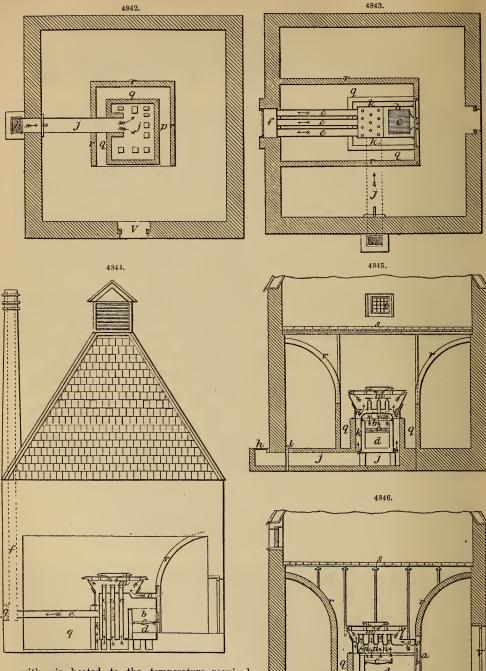
with air heated to the temperature required, which can be regulated at the will of the maltster. Pale malt requires but once turning on this kiln, and the difficulty of drying it is considerably decreased.
